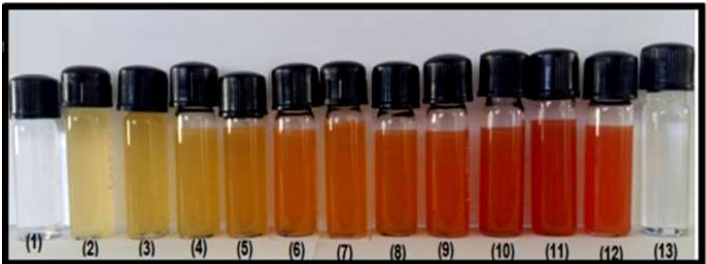
Figure 3. A photograph of test tubes of the culture of Providencia vermicola BGRW with different concentrations of \text{SeO}_2 and \text{CdCl}_2 to CdSe QDs production.
